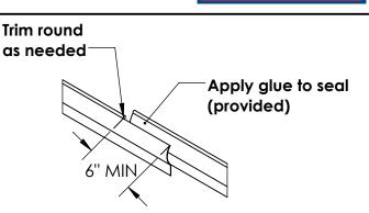
Once the weatherseal is fully wrapped around the perimiter, overlap the cut end and use glue to seal. Additional trimming may be necessary for proper fitment.
