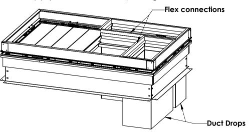
**<u>STEP 6</u>**: Install all duct supports provided with isolation rail using  $14 \times 1$ " Tek screws. locations and dimensions will be marked on submittal drawing.
